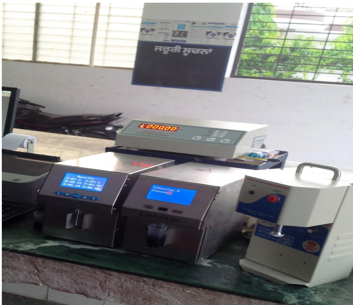
Photo 4.1 Fat and SNF measuring machine installed at VCS
